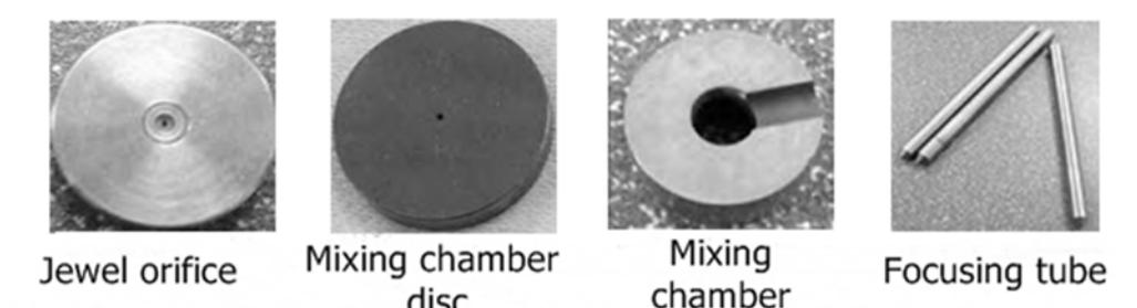
*Figure 7. Basic components of nozzle that need to be controlled during maintenance process [5].*
