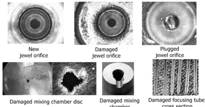
*Figure 8. Defects created on jewel orifice, mixing chamber disc, mixing chamber and focusing tube [5].*
