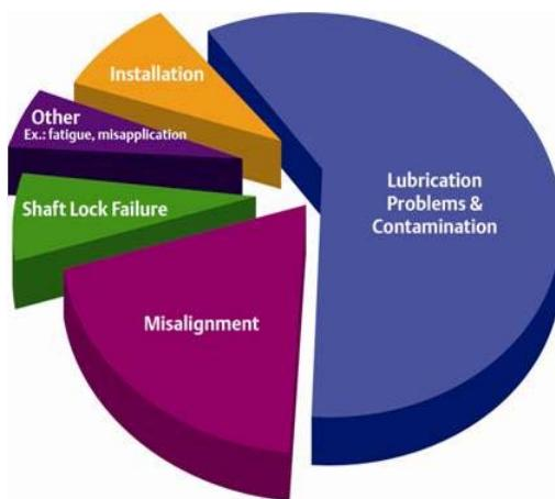
Lubrication is often organized according to someone's „feeling“, „until the grease goes out on the other side“ or using time tables as one exclusive criteria. There is a different way, proven to be better. On Condition Lubrication. This approach is considering fundamentals of level of friction and factors that influence it; speed, load, viscosity but also factors that we can not include in theoretical calculations to determine a time interval and quantity.
