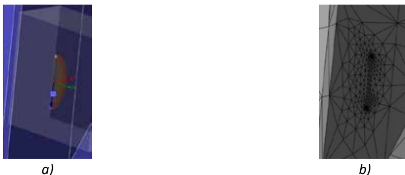
Figure 6. a) Local coordinate system and semielliptical crack and b) crack finite element mesh
