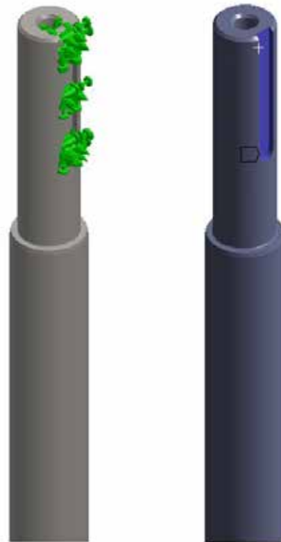
Figure 3 Fixed support in shaft frequency analysis - SolidWorks (left) and Ansys (right)
