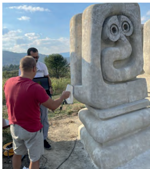
Slika 3. 3D skeniranje površine skulpture u hladovini skenerom Artec Eva Figure 3 3D scanning of sculpture surface in the shade with Artec Eva scanner
