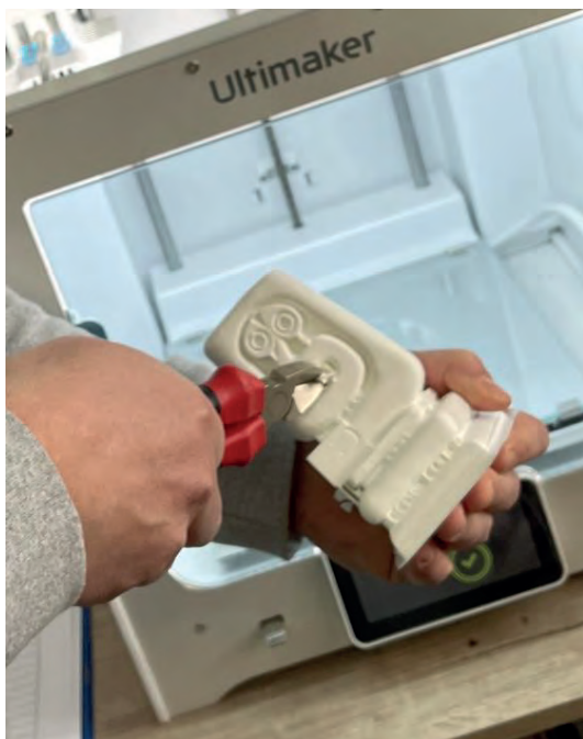
Slika 10. Uklanjanje potpora s replike skulpture Figure 10 Supports removal from a sculpture replica
