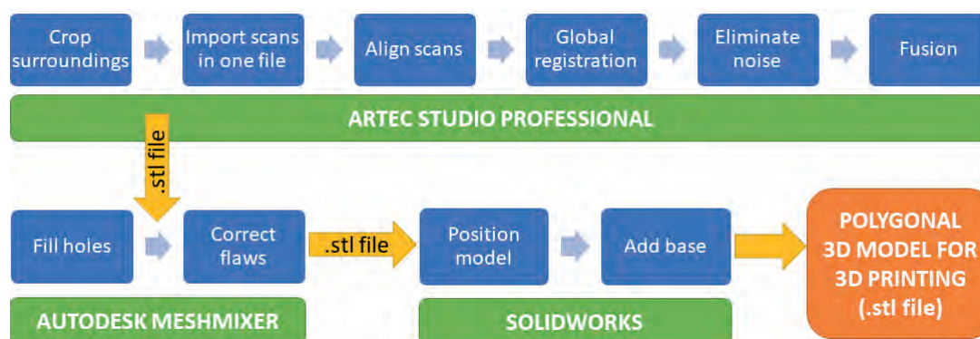
Slika 4. Proces obrade skenova i kreiranja 3D modela za štampanje Figure 4 Process of scans editing and creating the 3D model for printing
