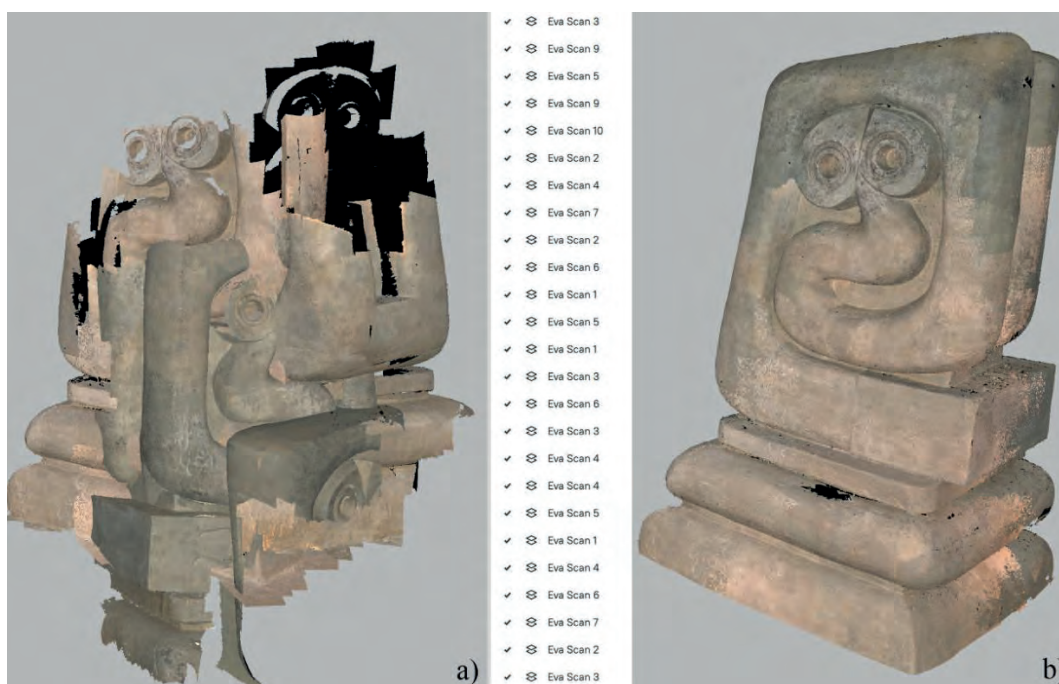
Slika 5. Artec Studio - obrada, neporavnati (a) i poravnati (b) 3D skenovi Figure 5 Artec Studio - editing, unaligned (a) and aligned (b) 3D scans
