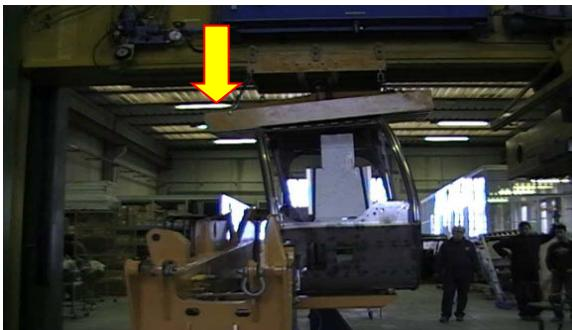
3. The structure of the cabin is then loaded with longitudinal force, whereby the starting direction of the load action should be horizontal and parallel to the longitudinal axis of the machine.
