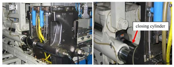
Figure 1. Closing unit together with tool (left) and closing cylinder (right)
