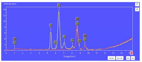
*Figure 4. Comparison of fresh (red spectrum, ISO 4406: 22/21/18) and used-up hydraulic oil (yellow spectrum, ISO 4406: >24/24/19*
