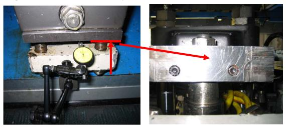
Figure 6. Incorrect adjustment of the support-screw (left) and strong signs of wear (right)
