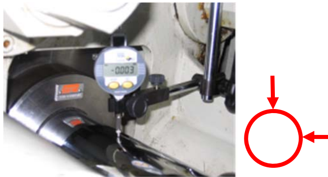
Figure 5. Motion accuracy measurement in two directions using precise gauge
