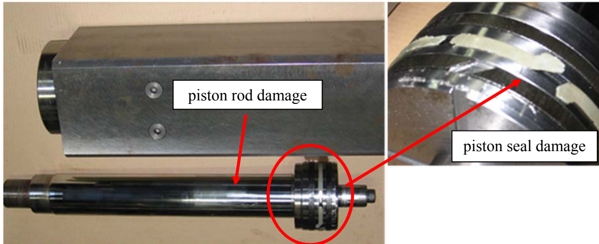
Figure 2. Damages on the piston rod and the seal
