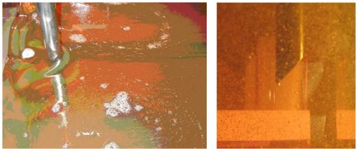
*Figure 3.* Foam on the surface of the oil (left) and air bubbles inside the oil(right)
