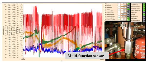
*Figure 4.* Integrated on-line multifunction sensor and graphical interface with the most important changes in the parameters
