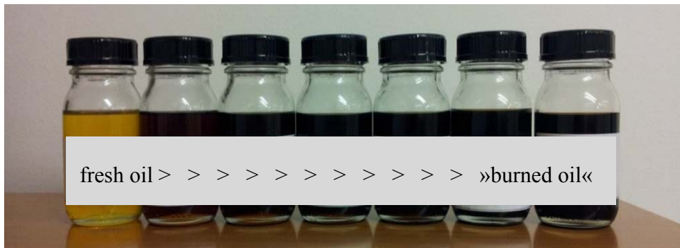
Figure 1. Rapid darkening of the oil in a short service period
