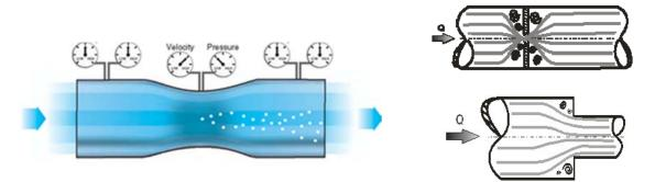
Figure 5. Pressure and speed conditions in tube with restriction causes air excretion
