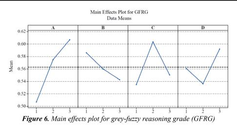
Based on Table 4 and Figure 6 the optimum setting of input process parameters is identified as cutting speed 162 m/min, depth of cut 1 mm, feed rate 0.214 mm/rev and workpiece material 42CrMo4, represented as  $A_3B_1C_2D_3$ . This is marked in bold font in Table 4. The use of these conditions will at the same time minimize *Fr* and *Ra* and maximize *MRR* throughout turning within the range of studied process parameters.
