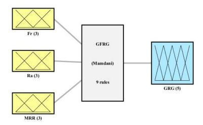
Figure 2. Structure of three inputs and one output fuzzy logic system
