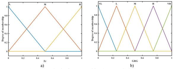
Figure 3. Membership functions used for: a) Fr input, b) GRG output
