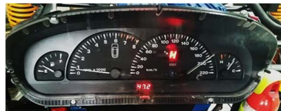
Figure 11 The control table with the speedometer, rpm meter, battery voltage display and gear position display (H as in Serbian Cyrillic neutral)
