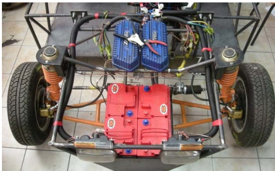
Figure 2 Front axle with in-wheel electric motors and batteries
