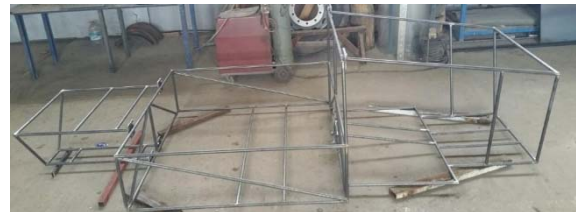
Figure 4 Tubular frame consisting of 3 modules in early stage of development
