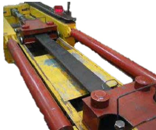
Figure 14. Vulcanized belt joint test
