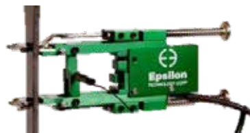
Figure 10. Elastic deformation test of a belt sample
