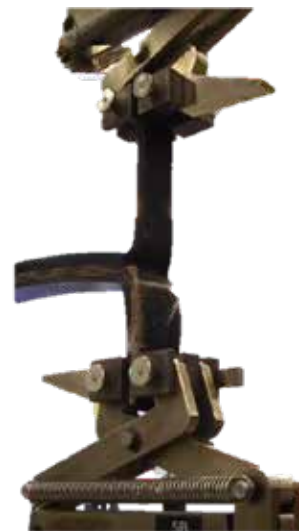
Figure 13. Test of resistance to layer separation of a belt sample
