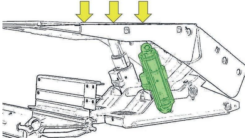
*Figure 1 Hydraulic cylinders as parts of roof rack*
