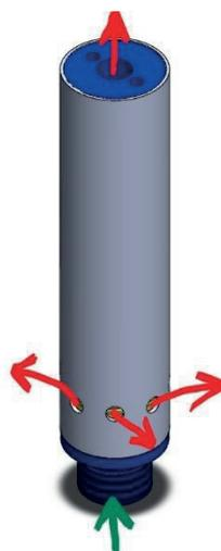
Figure 7 Entry and exit points of the fluid
