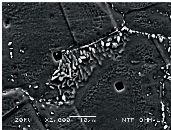
Figure 4 Microstructure by SEM of a sigma phase in an austenite stainless steel S21800 annealed at 850°C for 2 hours and water cooling, 2000x. Etched with aqua regia. [3]
