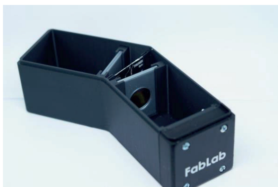
Slika 4.1 3D printani sklop spektrometra Figure 4.1 3D printed spectrometer assembly
