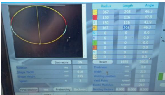
Figure 5 Example of entered parameters for ellipse transformation using two diameters
