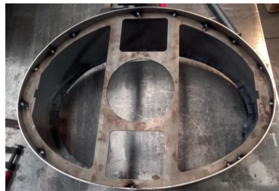
Figure 10 The final shape obtained by the transformation method using three diameters
