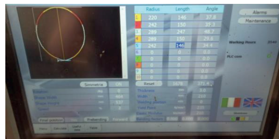
Figure 2 Example of entered parameters for arc length
