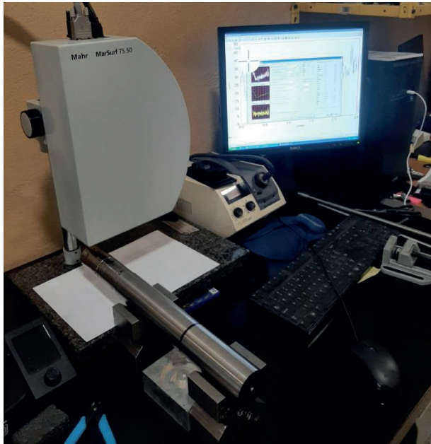
Figure 6 Mahr MarSurf TS 50 device during roughness measurement of the machined sample
