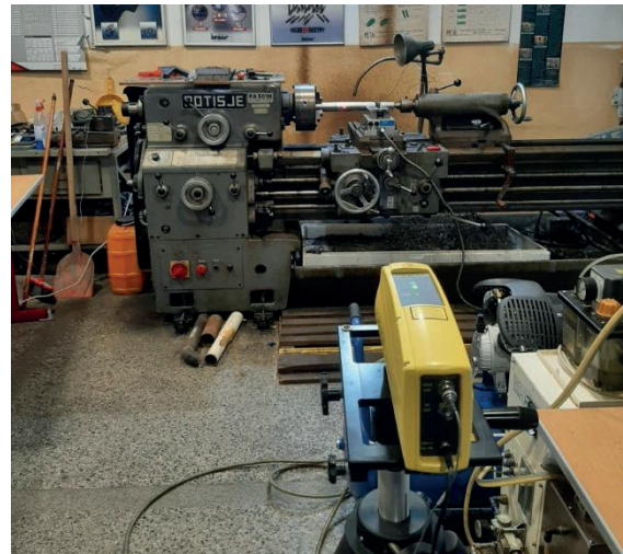
Figure 3 Ometron VQ-400-A Setup ready for vibration measurement
