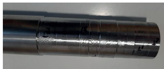
Figure 5 Appearance of the machined sample surface after the experiment
