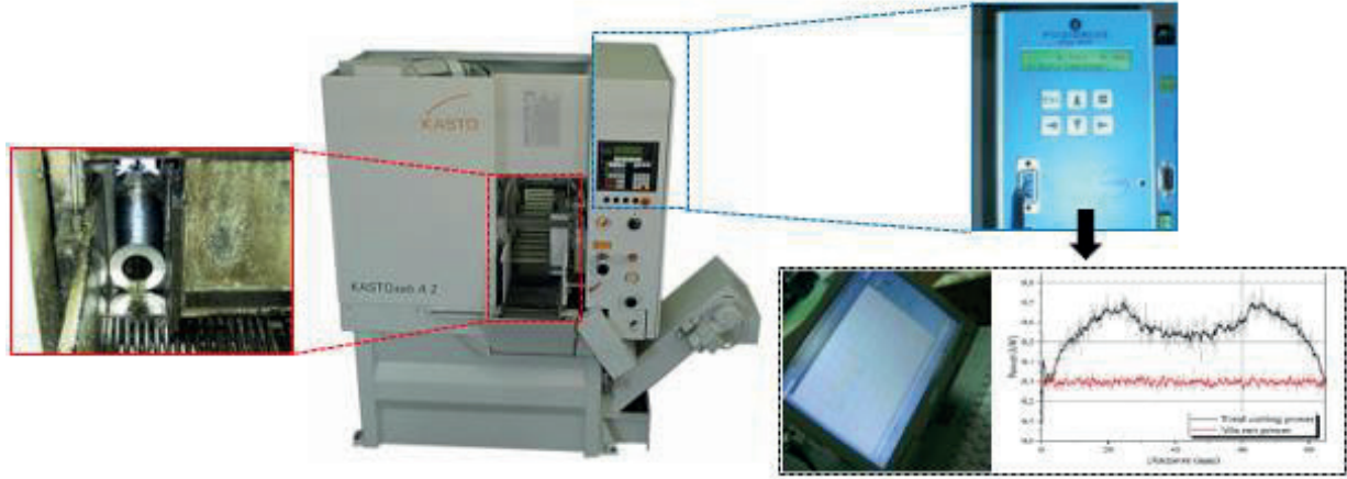
Figure 1 Experimental Setup of the Band Sawing Process
