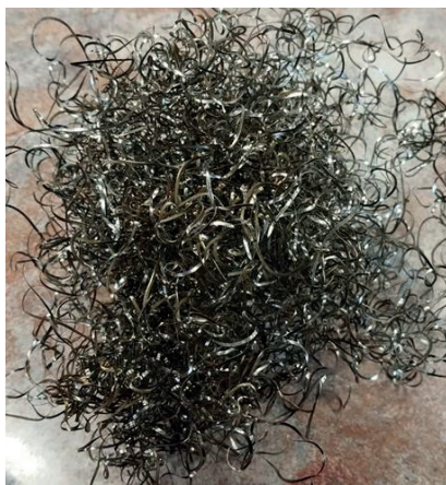
Figure 10. TA6V Chip that was formed after 30 seconds
