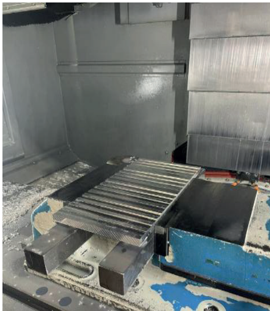
Figure 3 a) Display of the clamped semi-finished product and spindle milling cutter before the start of the experiment; b) AW 7075 plate after 16 passes
