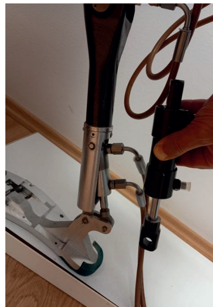
Figure 1. Cylinder of HP-FLUID d.o.o. Gradačac compared to the geometry of the prosthesis
