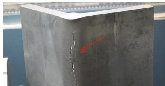
Figure 2. Cracks during air bending
