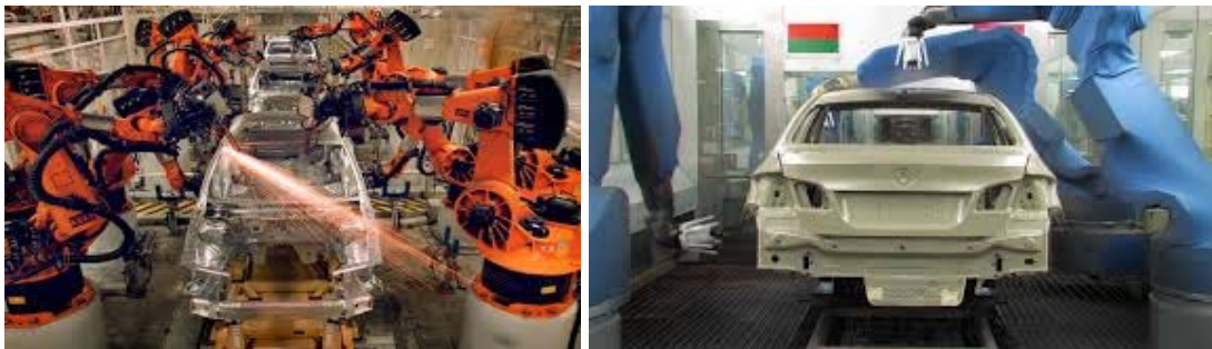
Figure 3. Application of industrial robots in the automotive industry [19,20]
