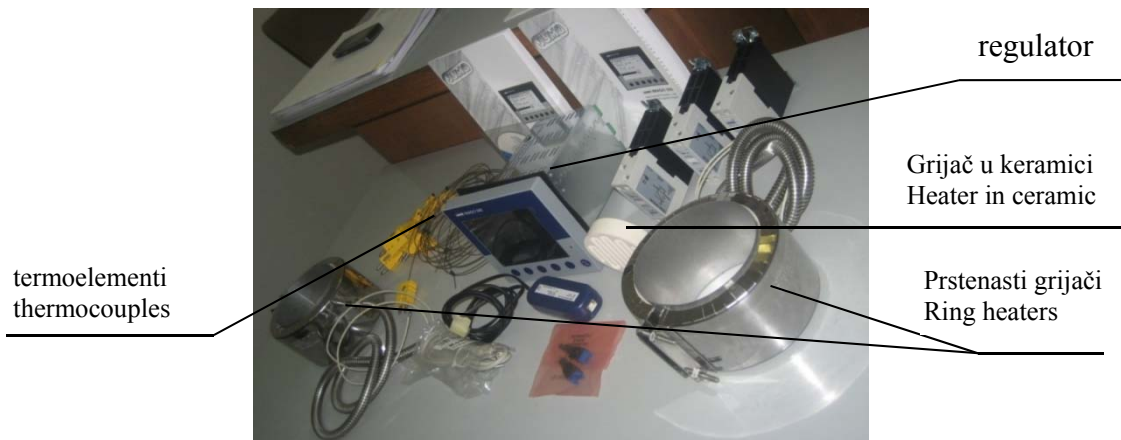
Slika 5. Termoelementi, grijači i regulator koji su u sastavu aparature Figure 5. Thermocouples, heaters and regulator that are part of the apparatus
