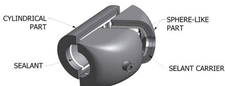
*Figure 2. Split sleeve for branch connection repairs*
