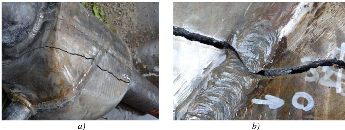
**Figure 10.** Position (a) and detail (b) of the crack after pressure test to destruction
