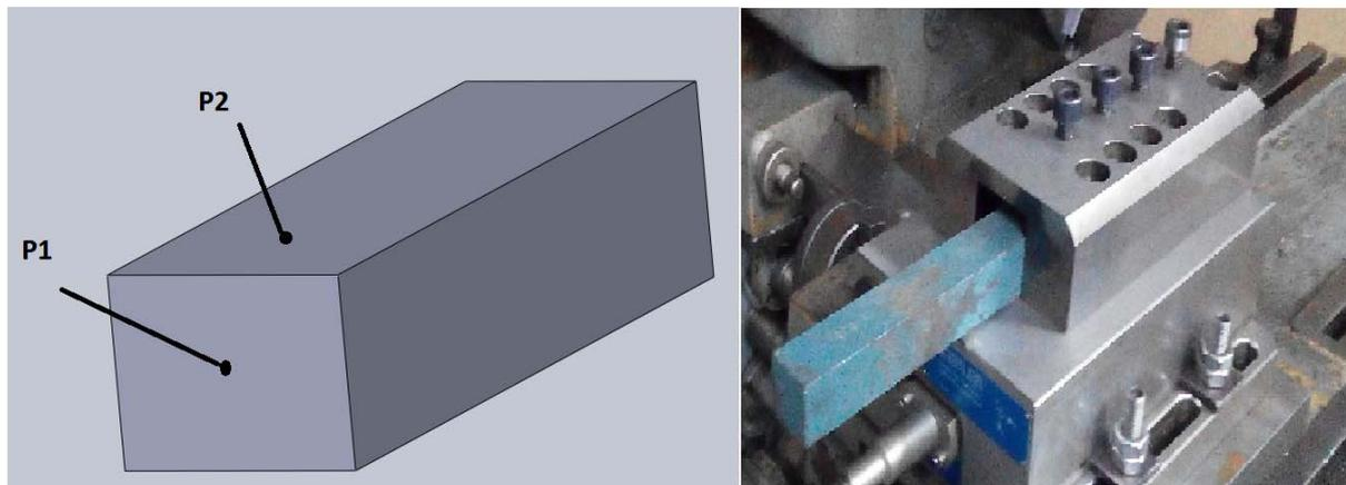
Figure 2. Kistler dynamometer with contact object mounted
