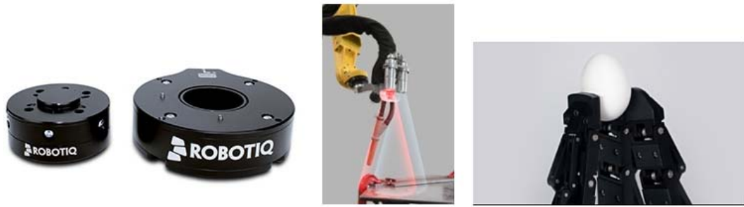
Figure 1. Different types of sensors: force/torque, vision and tactile.(from left to right) [4]
